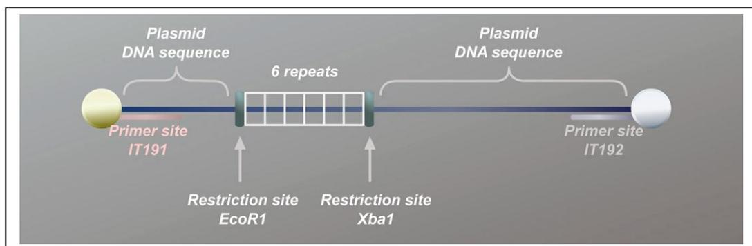
Figure 4: Components of single molecule substrate for use in molecular lithography.
